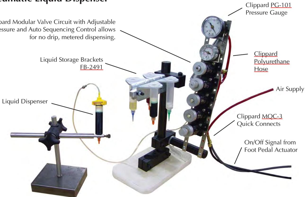
*This device precisely meters small amounts of liquids to parts with no drip or mess. It is made entirely of Clippard components.*
